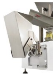
Stepper Motor operates the Weigh Bucket Gate
